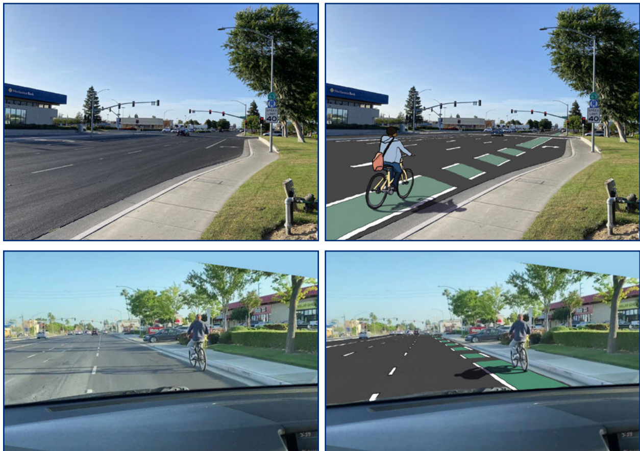
Figure 20: SR 63 Mooney Blvd Before and After the Project: Existing Design (left) vs. Proposed Design (right)
